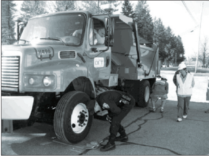
Figure 3-35: Trooper Huddleston (NH State Police) taking NHDOT wheel load measurements
