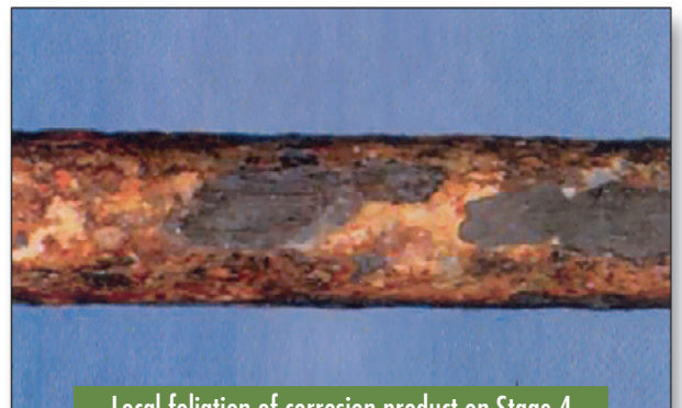
Local foliation of corrosion product on Stage 4
