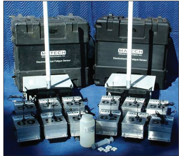
Figure 5-24: The EFS wireless access point antenna (back) with the numbered PDLs and individual wireless antennae (front). Sensors and electrolyte shown in foreground.
