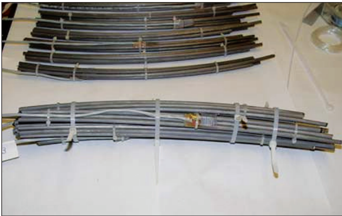
Figure 3-17: 49-Wire bundle to be placed in corrosion chamber
