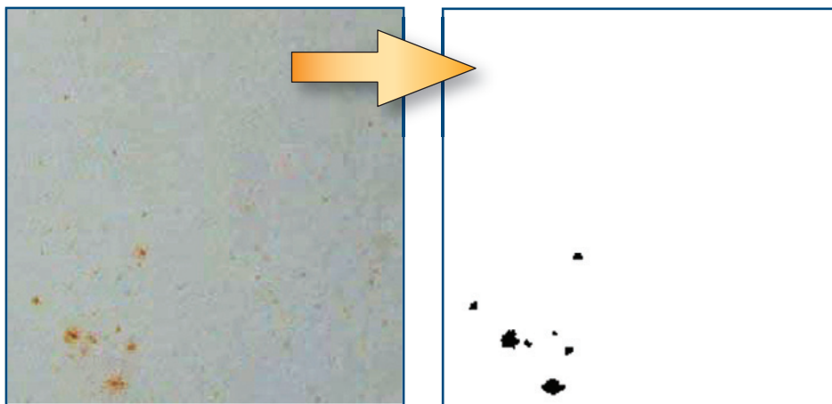
Figure 5-20: Processed Result under Non- uniform Illumination
