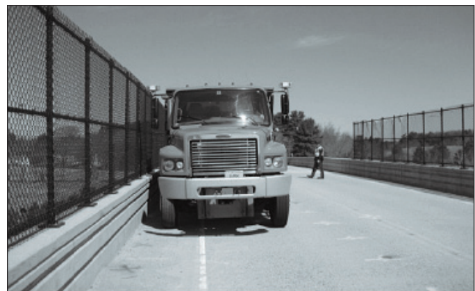
Figure 3-34: NHDOT sand truck as load application during April 2008 load test
