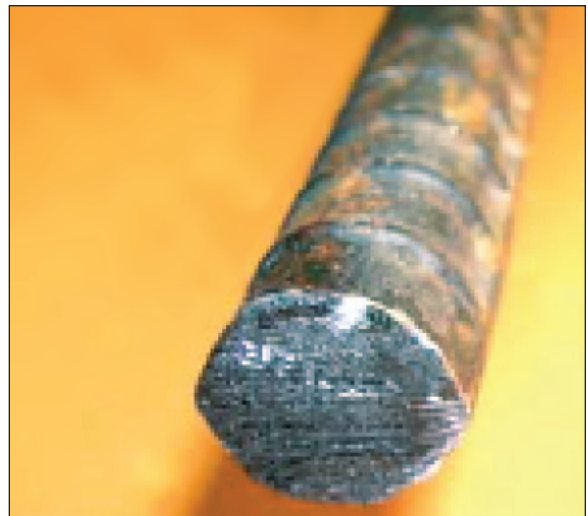
Figure 5-43: A typical rebar used for concrete reinforcement. Note the non-uniform cross-section.
