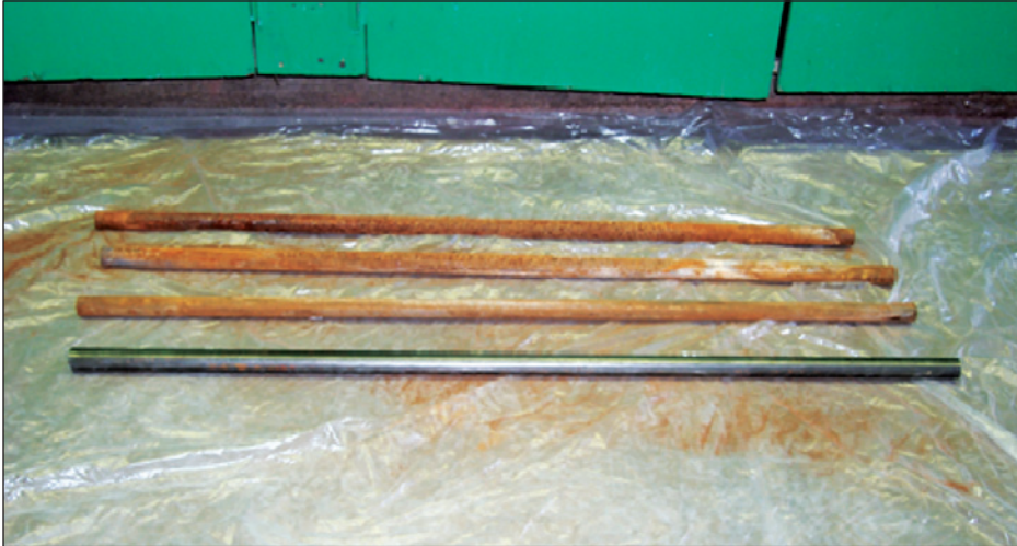
Figure 5-39: Four steel bars showing different degrees of corrosion – un-corroded case (bottom bar) to highly corroded case (top bar).
