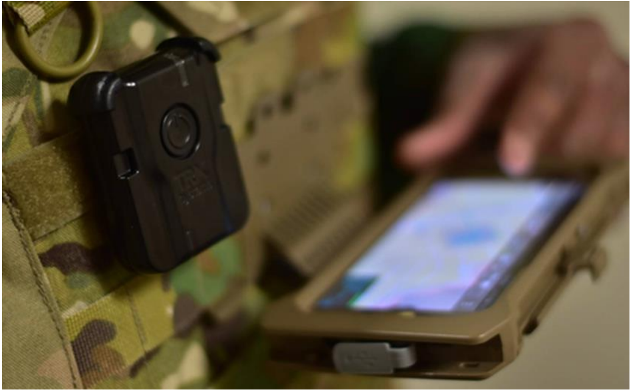
Figure 1-2 TRX NEON mounted on a tactical vest Image courtesy of TRX Systems
