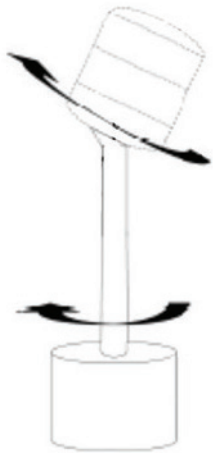
Diagram of an actuator including a mount and a rotator configured to mount a spinning sensor.
