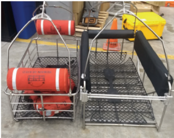
Photograph of the new improved rescue basket on the right next to the old USCG rescue basket on the left.
