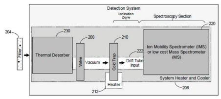
The detection system includes a thermal desorber and cold trap to collect and concentrate the vapor molecules and a low-cost detection system such as an IMS to detect contraband substances from Figure 3 of US Patent 11,709,149.
