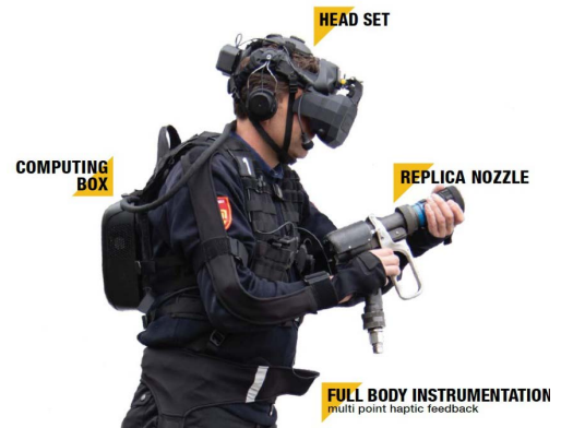
Figure 2-2 Computer-connected VR HMD with nozzle controller and haptic feedback
