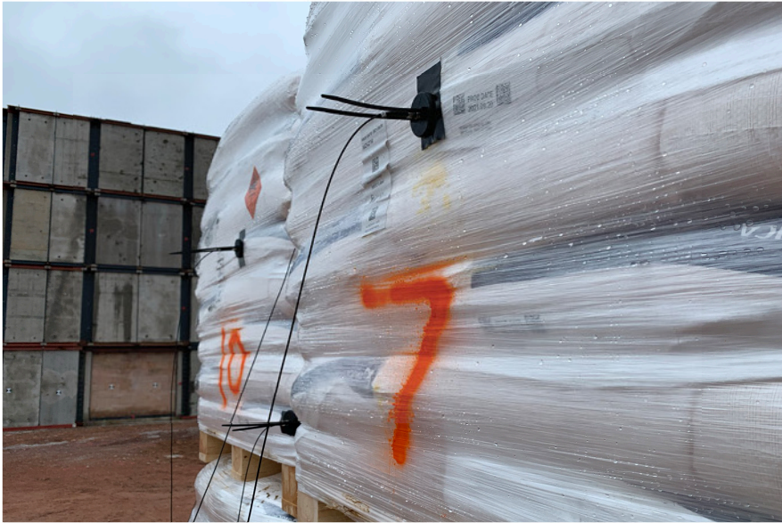
FLRS sensor assemblies embedded into explosives
