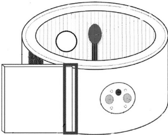
*Tourniquet gripper cuff featuring an electrical connection for the system and multiple sensors to collect patient vitals and monitor cuff pressure.*
