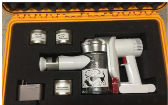
HVST-TED handheld sampling device, charging pack, and sampling traps in a hard case.
