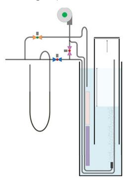
ICHV schematic depicting two nested cylinders, with the inverted cylinder holding an air chamber that is filled with an air supply line and drained with a line to a patient's inhalation tube. A third, shorter tube allows exhalations to be sent back to the water bath at a depth appropriate to provide back-pressure to guard against alveolar collapse. The manometer uses salt water or some other electrically conductive liquid to provide breathing signals from the patient to the control hardware.
