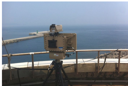
Figure 3-11 SR Hawk Surveillance Radar
