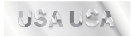
Microprinted embossing plate design, showing each character partitioned into a mix of tactile and matte elements, shown in Figure 72 of US Patent Application 17/961,951.
