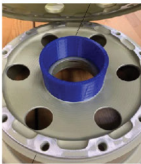
SWMA seal fitted to a wheel bearing of a landing gear wheel assembly. The second wheel bearing would be placed on top of the seal to enclose the space between the two wheel bearings.
