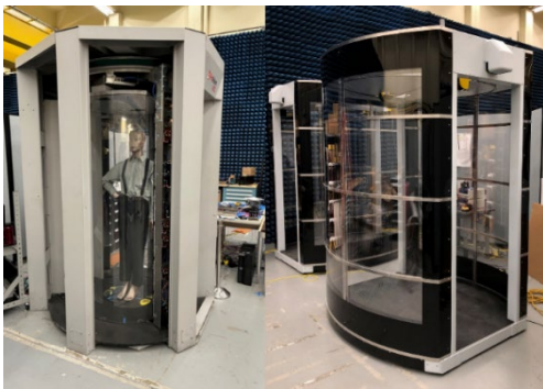
High Definition-Advanced Imaging Technology retrofit kit (left) and the passenger screening portal (right). Photo Credit: PNNL
