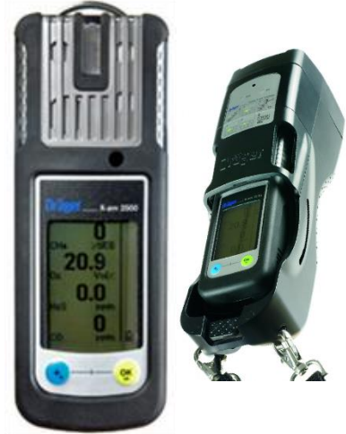
Left image is the X-AM 2500, the right image shows the sensor in the optional pump
