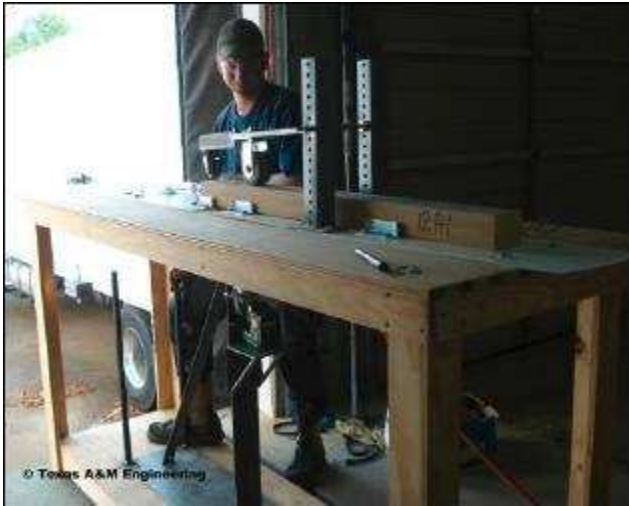
Figure 1. Bench test apparatus for testing cordless reciprocating saws.
