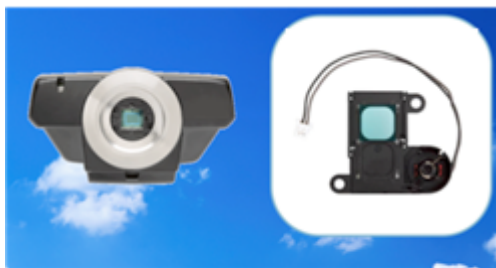
Figure 5: Day/Night Camera Imager IR Cut Filter Engaged
