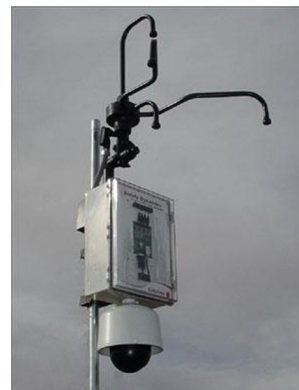
Acoustic Sensor Unit with Multiple Microphones and Integrated Camera
