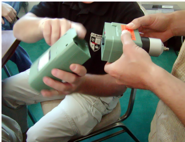
Figure 3-9. Changing PID Batteries
