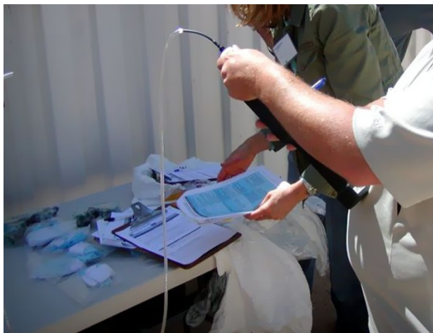
Figure 3-6. Drawing Sample Through 6-Foot Tube
