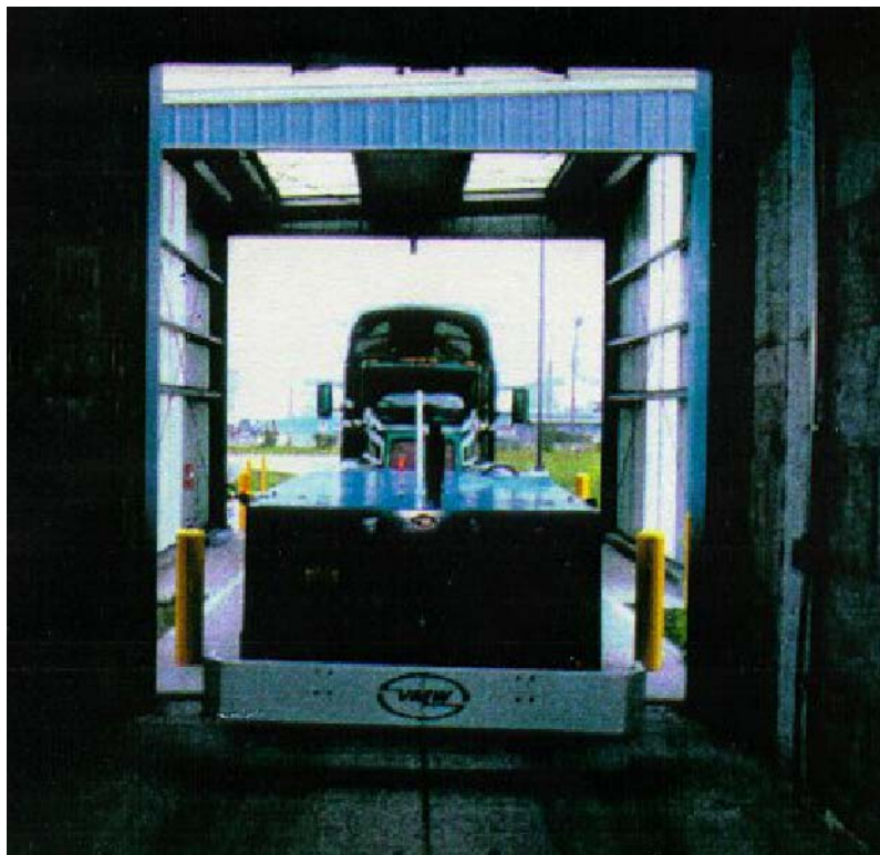
Figure 11. Via remote control, the AGV guides the tractor-trailer through the Inspection Building.
