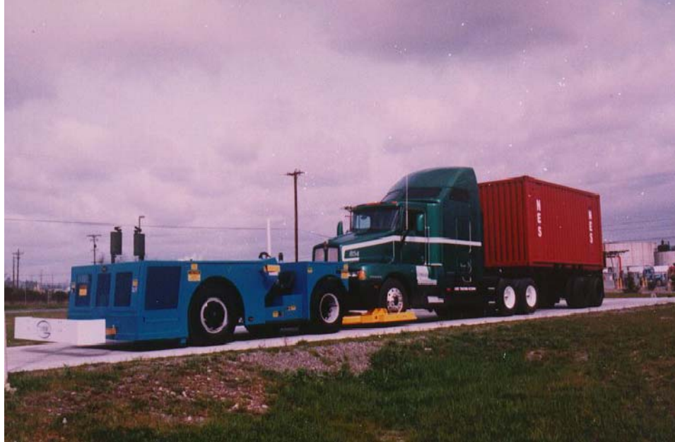
Figure 10. The AGV tows a truck by its front wheels.
