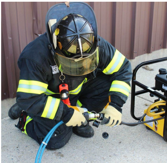
A firefighter connects a hydraulic hose to an extrication tool using prototype structural firefighting gloves during the operational field assessment held at NIPSTA in Glenview, Illinois.
