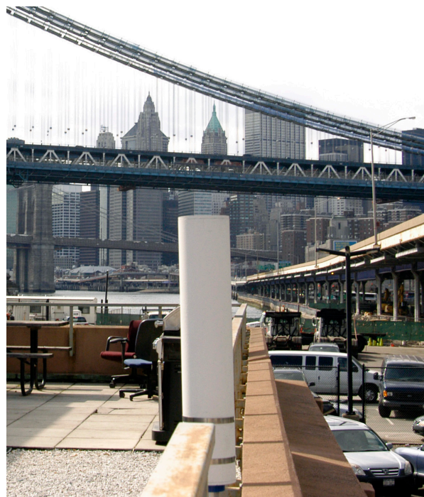
REMS sensor installation in New York City.
