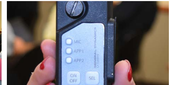
Communications hub device which integrates an array of wireless communications technologies including land mobile radios, smartphones and WiFi.
