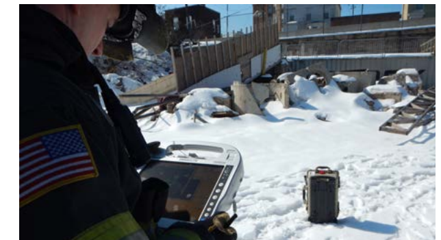
Newark Search and Rescue Firefighter operating FINDER on a rubble pile to locate victims during the OFA.
