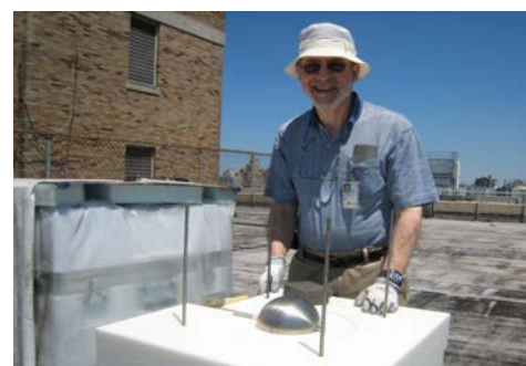
NUSTL Physicist Paul Goldhagen disassembling the largest of the 16 detectors of the Laboratory's extended-range multisphere neutron spectrometer after completing the long-term measurement of background neutrons made on NUSTL's roof.
