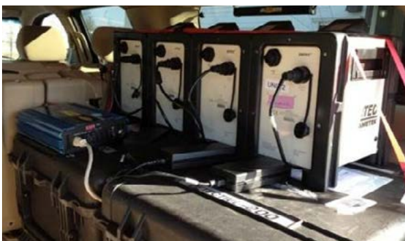
SRD mounted in the trunk of a sport utility vehicle
