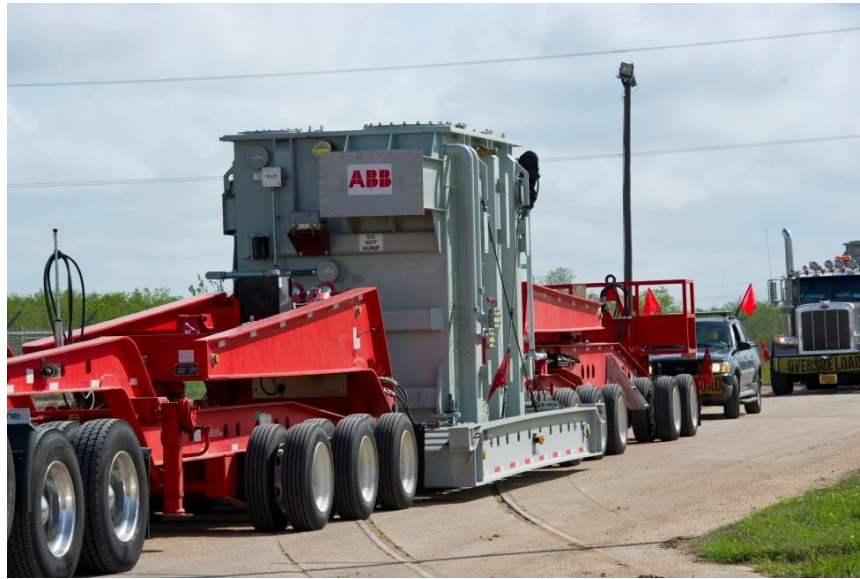
Figure 3. Transportation of the Recovery Transformer on the MA-65 custom trailer avoids the need to prepare a special surface or lay concrete at the substation prior to deployment.
