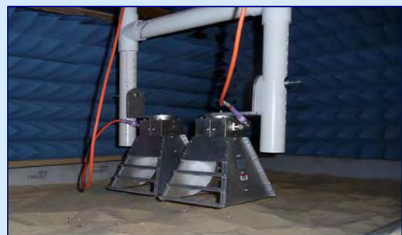
Groundbreaking: An early prototype of S&T's ground-penetrating radar on display at a demonstration. Engineers tested the technology in a giant sandbox to simulate conditions along areas of the southern U.S. border.
