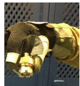
Figure 3-12 Length of Glove C Fingertips Surpassing First Knuckle during Dexterity Activities
