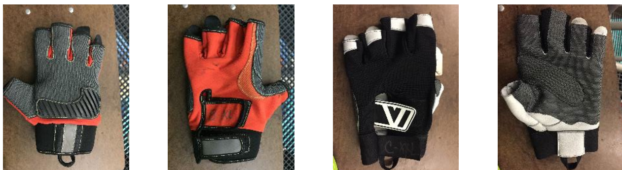
Figure 3-4 Sample of Glove B (Left) and Glove C (Right) Following Degradation Testing
