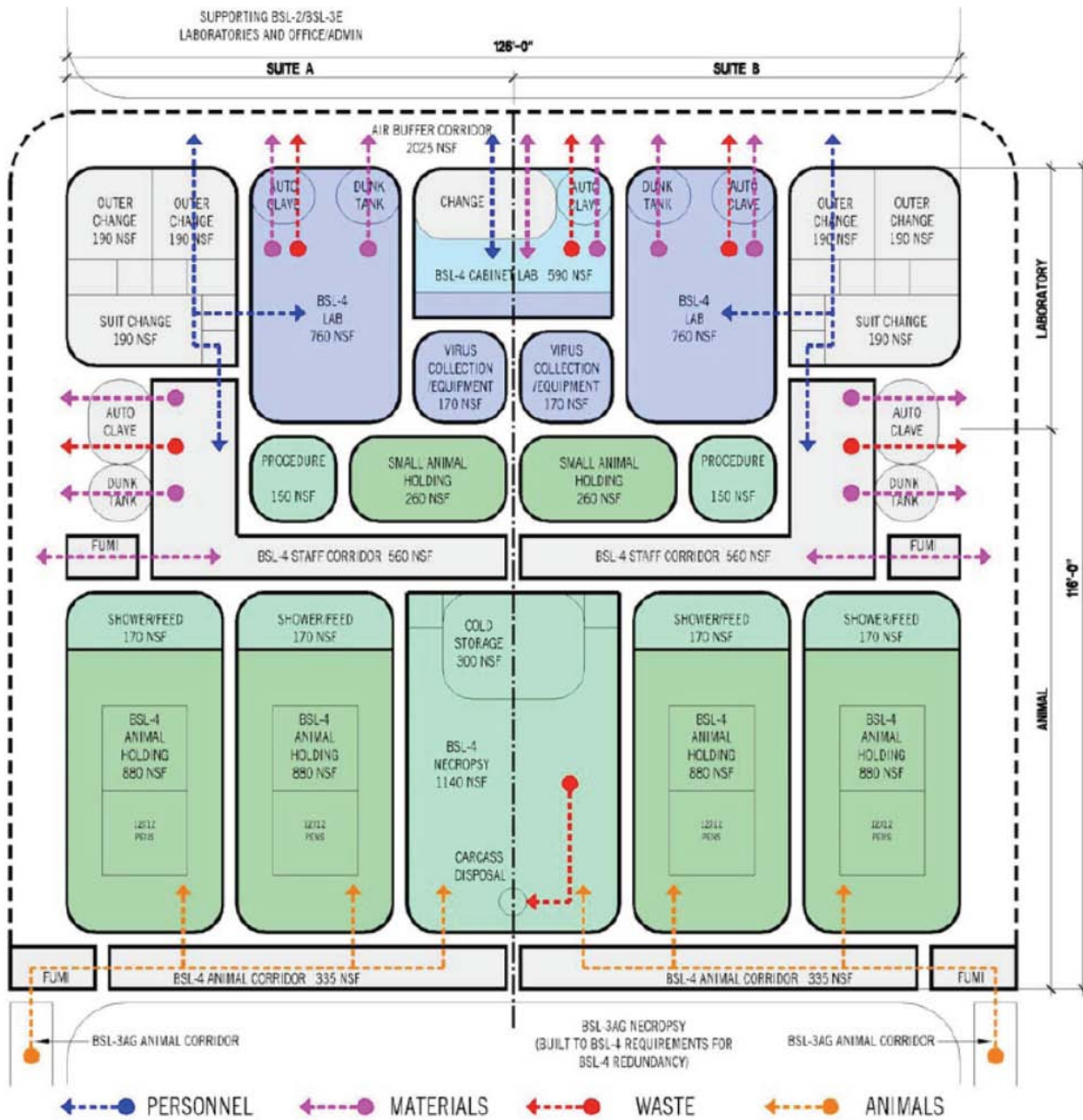
Figure E.2.2.2-3 — NBAF BSL-4 Process Flow Diagram (NBAF 2007)
