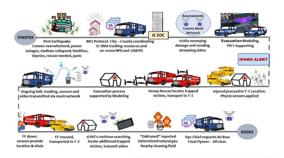
Summary: Post-earthquake: Comms overwhelmed and power outages. On-scene sUASs used to locate victims, provide SA & comms mesh networks. MCI declared, additional resources requested. sUAS and camera providing SA. Sensors monitoring responder locations & patient vitals. Comms repeaters transmit sensor and video data from stadium. Firefighters and victims rescued and directed to T-3. Gas/chem sensors alert of potential hazards in stadium.
