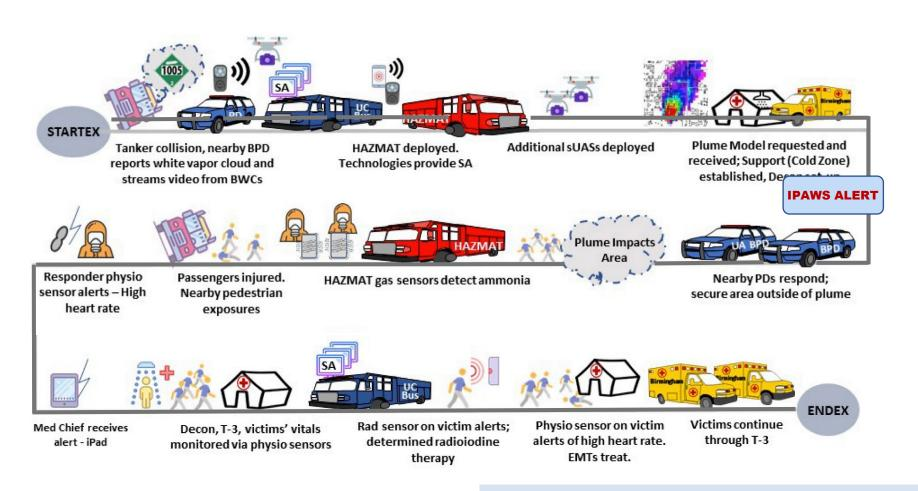
Summary: Collision causes HAZMAT incident on stadium grounds. Various video systems provide situational awareness. Vapor cloud impacts area. HAZMAT arrives, plume model received, zones established, decon set-up. HAZMAT detects ammonia when approaching the tanker,. Pedestrians proceed through decon. Radiation detected on one victim. Physio sensors applied and alerts of high heart rate on victim. Victims proceed through T-3.
