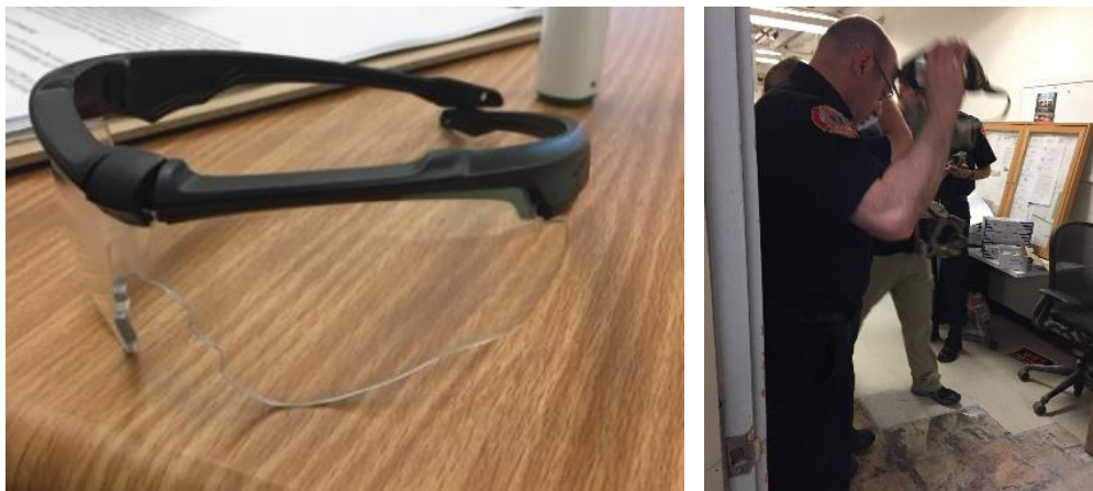
Figure 3-8 Assessing Durability Spectacles After Being Folded Inward (Left); First Responders Conducting Durability Testing on Goggles (Right)
