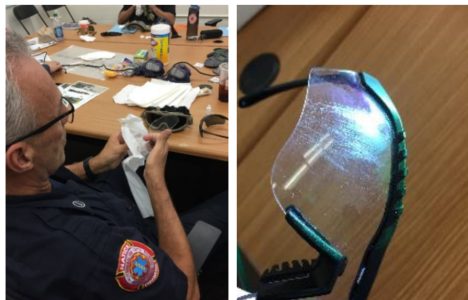
Figure 3-6 Assessing Scratch Resistance First Responder Attempting to Scratch Lenses (Left); Spectacles Following Scratch Resistant Testing (Right)
